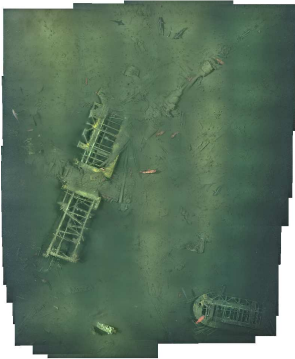
Figure 8: High-resolution post-processed photomosaic of the hangar portion of the Macon wreck showing the remains of two of the Sparrowhawk airplanes on board the airship when it went down. The high-resolution mosaic is based off a \sim 8 \text{ m} \times 12 \text{ m} portion of the real-time mosaic, containing \sim 100 images.
