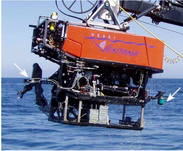
Figure 2: The MBARI ROV Ventana . Arrows highlight the primary sensors used in the real-time mosaicking and navigation system: a downward-looking video camera mounted on an arm at the front of the vehicle, and a DVL mounted at the rear.
