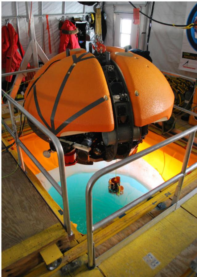
**Fig. 2** The AUV ready for deployment down the melt hole. To ensure that the AUV had sufficient energy reserves for each mission, it was kept on charge through the sonde calibration cycle. The vehicle was then lowered into the water, the sonde 'homed', and the charging cables freed to allow it to begin its journey
