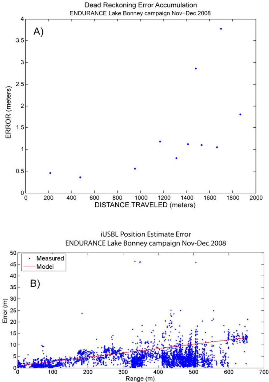
**Fig. 3** ENDURANCE performance at WLB in 2008: (A) dead-reckoning navigation error as a function of distance travelled as determined upon return to the melt hole in 2008, where the  $1\sigma$  error was 0.13 per cent of the distance travelled; (B) iUSBL navigation error as a function of range from transponder where the  $1\sigma$  error was  $0.9\text{ m} + 0.019 \times \text{range}$
