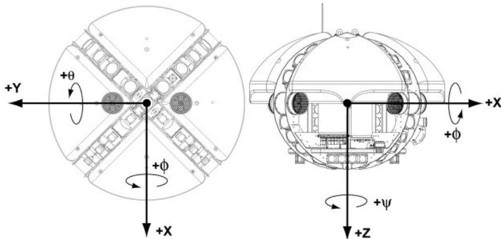
**Fig. 1** Vehicle-centric coordinate system for DEPTHX. The overall diameter (major ellipsoid axis) is 2.13 m and the height (ellipsoid minor axis) is 1.52 m. The vehicle dry mass in air is 1272 kg. It is neutrally buoyant under water
