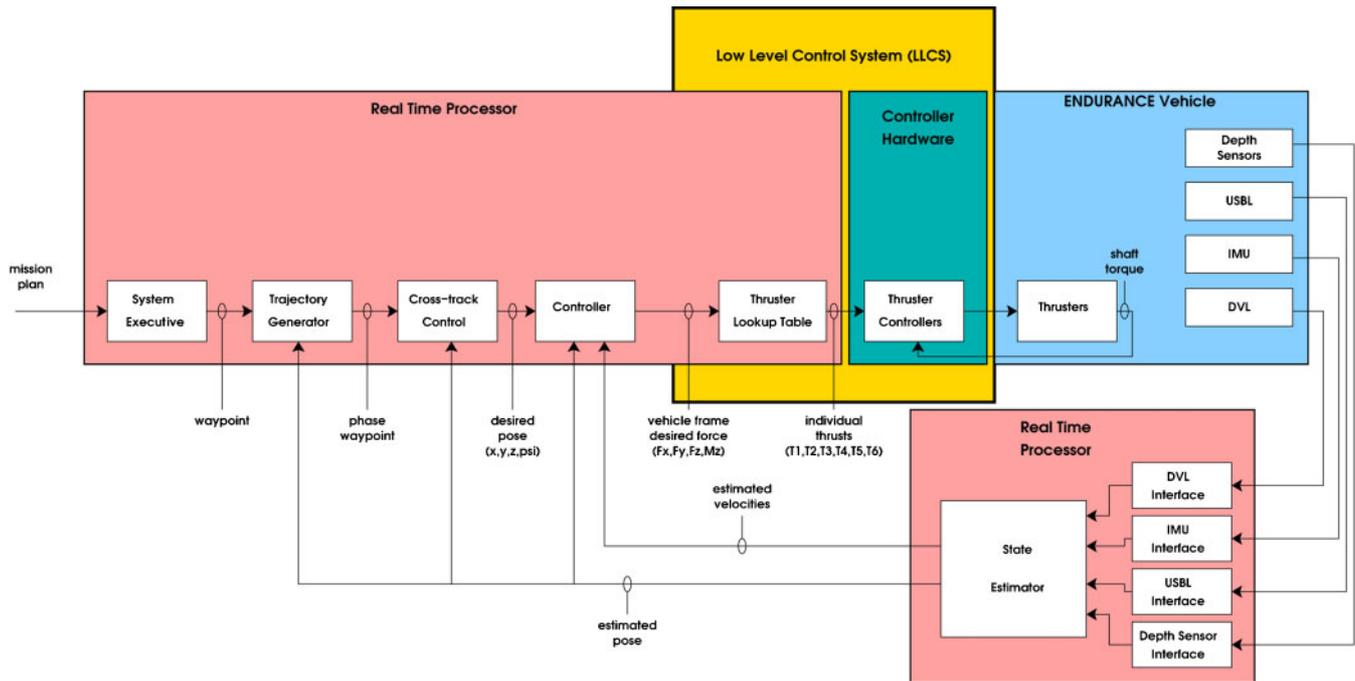
Fig. 4 ENDURANCE control system for under-ice transit and station keeping
